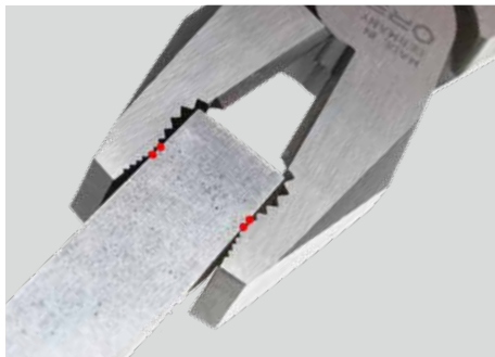
4-Punkt-Evolventen-Brennerloch 4 point involute pipe hole
